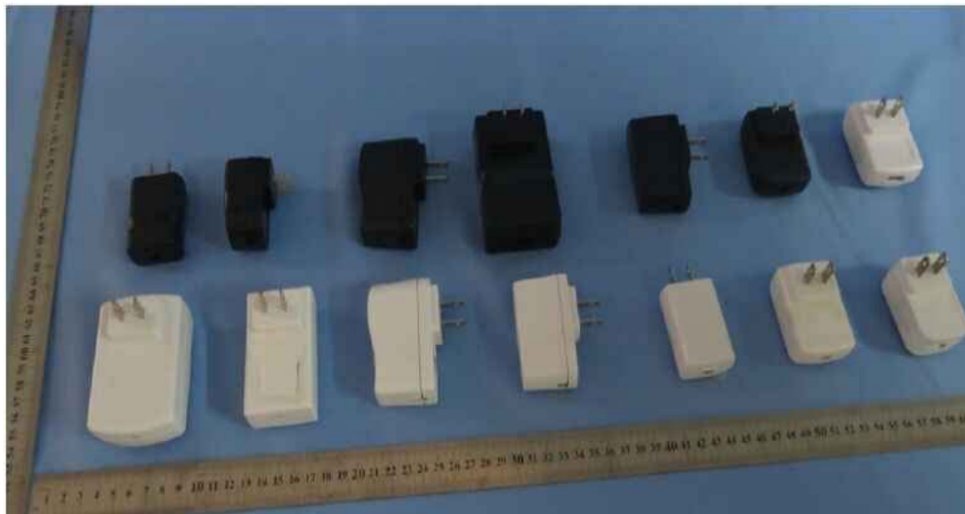
Photo 1 Before Glow-wire Test
