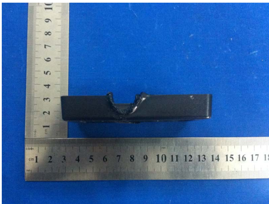
Photo 4 After Glow-wire Test
